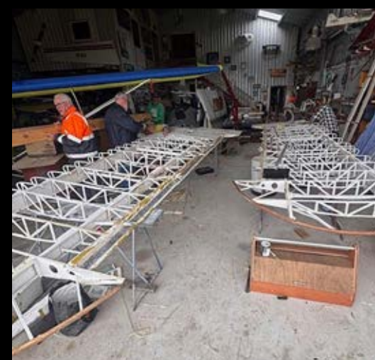
Beverley Soaring Society (below) Beverley's Pawnee tug ALA's wings getting refurbished (and a new spar) down in Albany.
